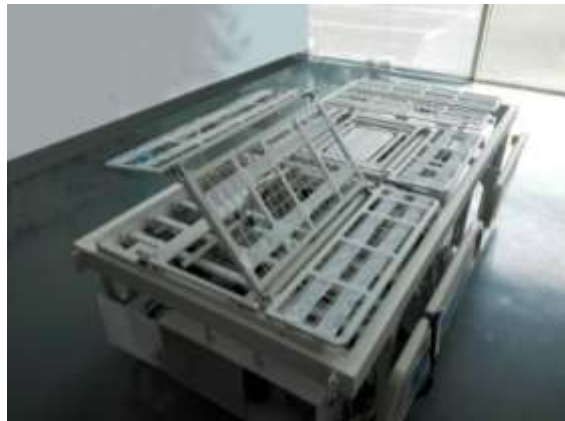
Figure 3-4 Picture of real Nursing bed frame turning to the right
